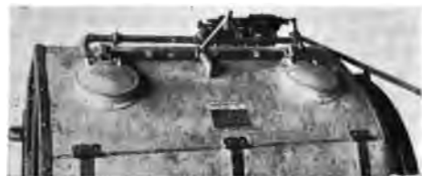
Fig. 7. Automatic Steam Connection for Drying Tumblers.
